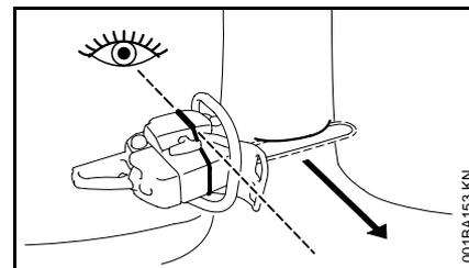
When making the felling notch, use the gunning sight on the shroud and housing to check the desired direction of fall:
