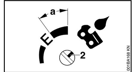
Oil pumps with a slot (2) in the adjusting screw: When the pump is set to range "a", the oil tank may run dry before the fuel tank and the chain will not be lubricated.
