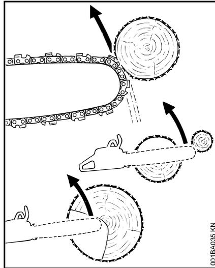
The reaction of the cutting force of the chain causes a rotational force on the chainsaw in the direction opposite to the chain movement. This may fling the bar up and back in a lightning fast reaction in an uncontrolled arc mainly in the plane of the bar. Under some cutting circumstances the bar moves towards the operator, who may suffer severe or fatal injury.
