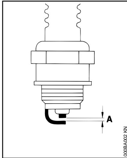
Wrong fuel mix (too much engine oil in the gasoline), a dirty air filter and unfavorable running conditions (mostly at part throttle etc.) affect the condition of the spark plug. These factors cause deposits to form on the insulator nose which may result in trouble in operation.
