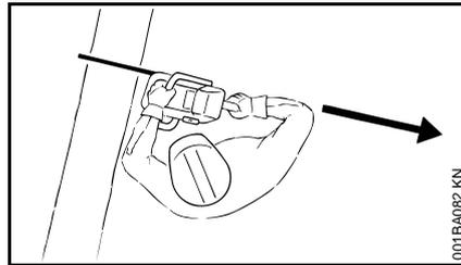
Position the chainsaw in such a way that your body is clear of the cutting attachment whenever the engine is running. Stand to the left of cut while bucking.
