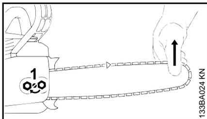
Retensioning during cutting work:
