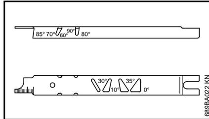
Use a STIHL filing gauge (special accessory – see table "Sharpening Tools"). This is a universal tool for checking the filing and side plate angles, depth gauge setting and cutter length. It also cleans the guide bar groove and oil inlet holes.
