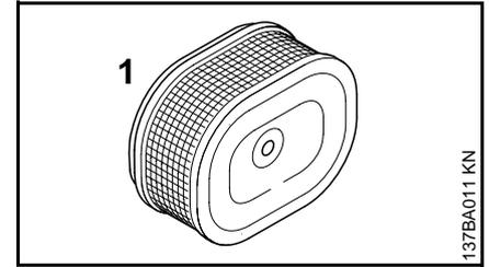
**Standard** wire mesh filter (1) (green) for normal normal operating conditions and winter operation.
