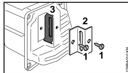
If the engine is down on power, check the spark arresting screen in the muffler
